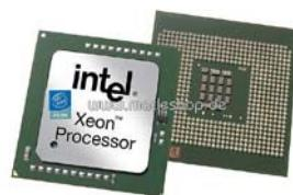
The main unit inside the computer is the CPU. This unit is responsible for all events inside the computer. It controls all internal and external devices, performs arithmetic and logic operations. The CPU (Central Processing Unit) is the device that interprets and executes instructions.
